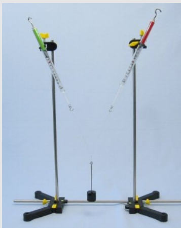
Load aligned force gauges with weight plate
