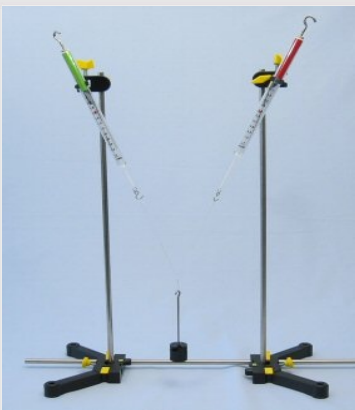
Test setup for determining the parallelogram of forces
